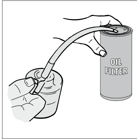
22 Oiling the oil seal
